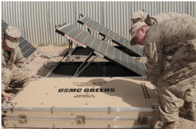
US Marines deploying portable solar/battery units
