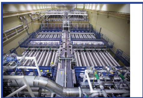
NIF Laser Bay--Seen from above, each of NIF's two identical laser bays has two clusters of 48 beamlines, one on either side of the utility spine running down the middle of the bay. Credit: Lawrence Livermore National Laboratory
